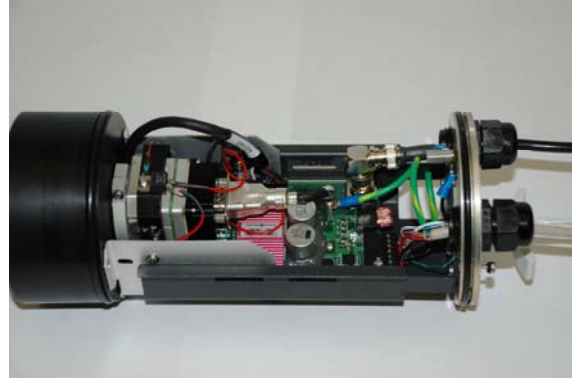
Figure 2-3: SR-309 Camera with and without the Environmental Enclosure
