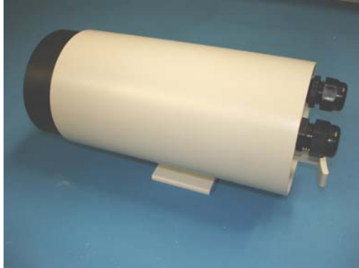
Figure 2-3: SR-309 Camera with and without the Environmental Enclosure
