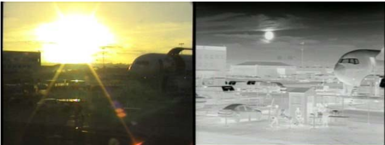
Figure 3: Backlit daylight camera on left; thermal camera on right
