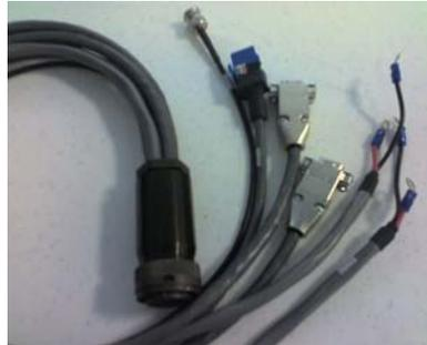
**Figure 5:** Break-Out Connector Cable
